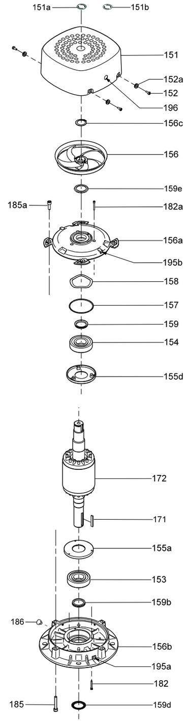
Fig. 22 Detail from fig. 29, exploded view of the MGE-F
