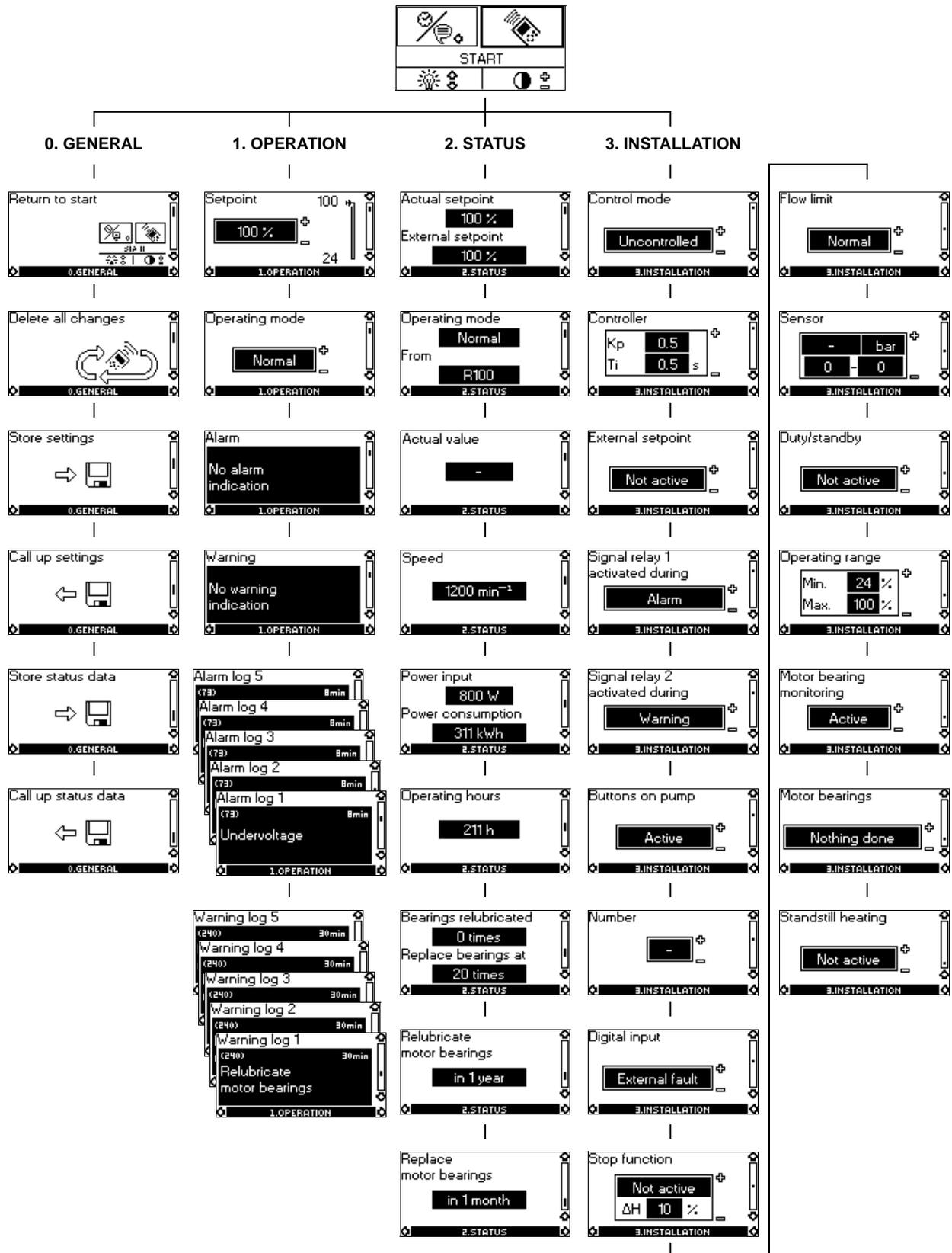
Fig. 16 R100 menu structure (for CRE pump)
