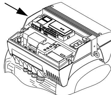
Fig. 6 Position of configuration label
