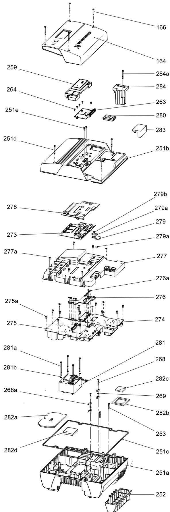
Fig. 30 Exploded view, terminal box
