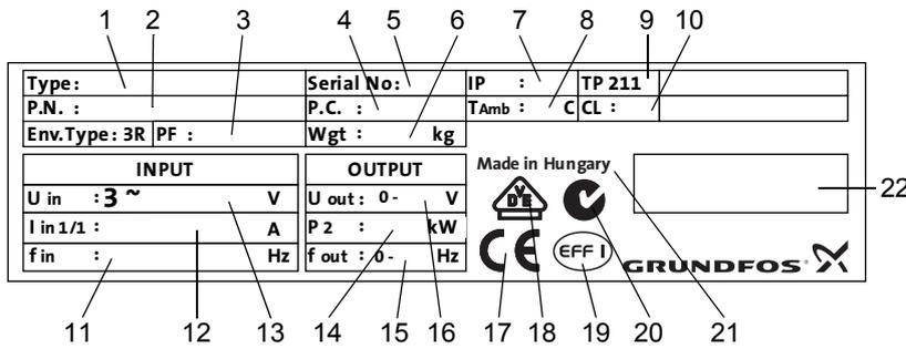
Fig. 1 Nameplate for MGE-F, efficiency 1 motor
