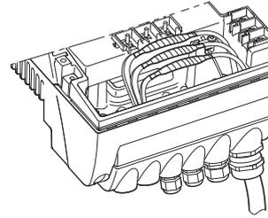
Fig. 28 The joints placed in the terminal box
