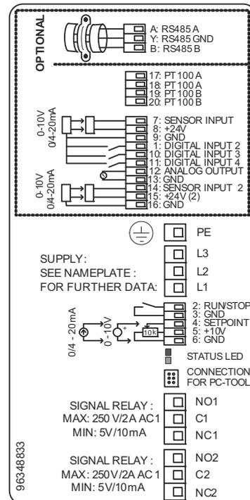
Fig. 9 Extended I/O module and GENibus
