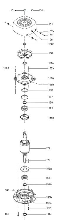
Fig. 20 Detail from fig. 29, exploded view of the MGE-F
