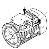
Fig. 4 Position of motor nameplates
