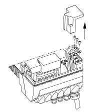
Fig. 23 Cover over the supply terminals
