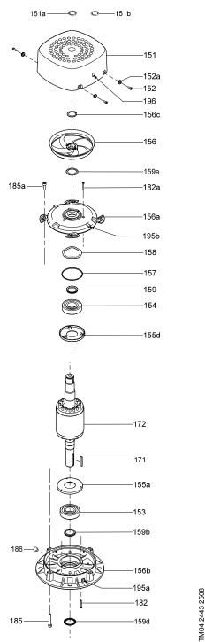
Fig. 22 Detail from fig. 29, exploded view of the MGE-F
