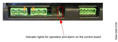
Fig. 14 Indicator lights inside the terminal box
