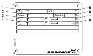
Fig. 31 Lubricating plate of MGE-F
