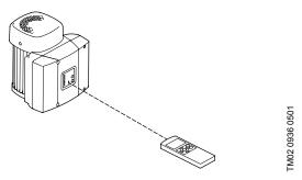
Fig. 15 The R100 communicates with the motor via infrared light
