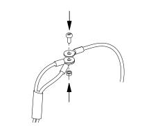
Fig. 26 Joining the motor conductors (two) and the supply conductor
