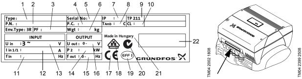
Fig. 1 Nameplate for MGE-F, efficiency 1 motor
