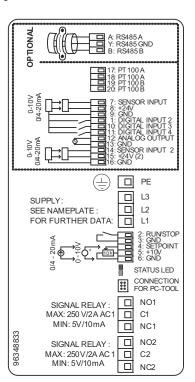
Fig. 9 Extended I/O module and GENIbus
