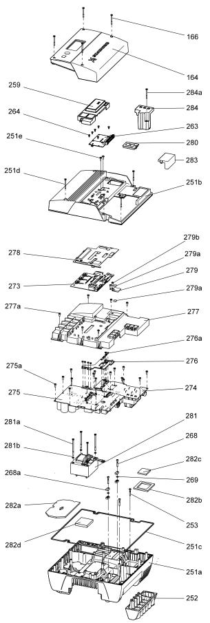
Fig. 30 Exploded view, terminal box
